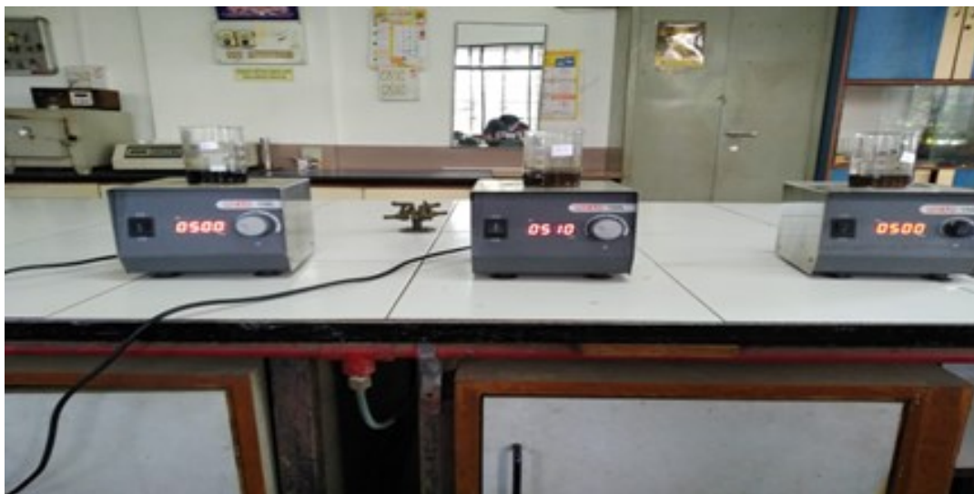
Figure 1: Magnetic Stirrer for Stirring Nanofluid. (PES's MCOE Chemistry lab)
